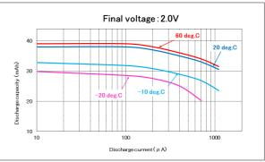
\* Nominal capacity indicates duration until the voltage drops down to 2.0V when discharged at a nominal discharge current at 20 deg. C.
