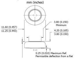
0.08 (0.003) Minimum Ref. (applies to top edge of gasket or edge of crimp, whichever is higher)
