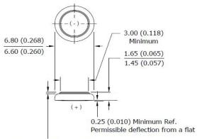
0.02 (0.001) Minimum Ref. (applies to top edge of gasket or edge of crimp, whichever is higher)
