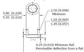
0.02 (0.001) Minimum Ref. (applies to top edge of gasket or edge of crimp, whichever is higher)
