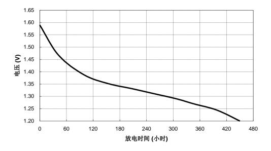
Discharge method: 33k $\Omega$ , 24hours/day, E.V. 1.2V Temperature: 20±2 $^{\circ}$ C
