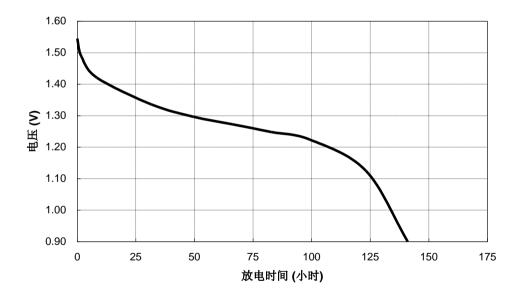
Discharge method:  $6.5k\Omega$ , 24hours/day, E.V. 0.9V Temperature:  $20\pm2^{\circ}$ C
