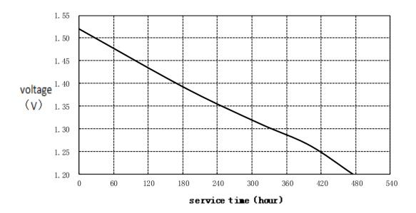
Discharge method: 47k $\Omega$ , 24hours/day, E.V. 1.2V Temperature: 20±2 $^{\circ}$ C
