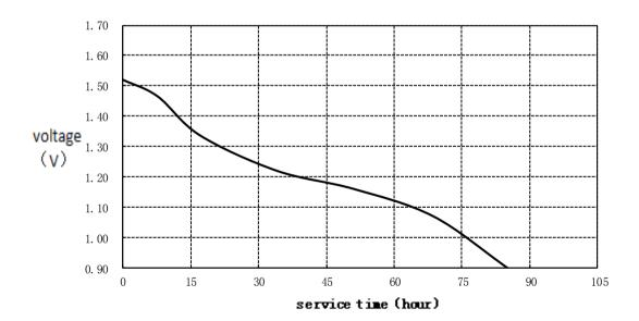
Discharge method:  $6.5k\Omega$ , 24hours/day, E.V. 0.9V Temperature:  $20\pm2^{\circ}$ C
