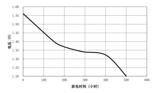
Discharge method:  $68k\Omega$ , 24hours/day, E.V. 1.2V Temperature:  $20\pm2^{\circ}\mathbb{C}$
