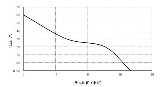
Discharge method:  $6.5k\Omega$ , 24hours/day, E.V. 0.9V Temperature:  $20\pm2^{\circ}$ C
