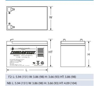
Tolerances are +/- 0.04 in. (+/- 1mm) and +/- 0.08 in. (+/- 2mm) for height dimensions. All data subject to change without notice.
