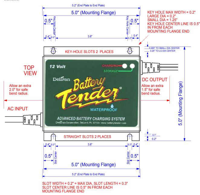
**Caution** – It is possible that part of the charger outer case may reach as high as  $70^{\circ}$  C ( $158^{\circ}$  F) during normal operation, delivering full power. More than likely the maximum case temperature will be only about  $50^{\circ}$  C ( $122^{\circ}$  F). However, it is important that the charger is located in an area with adequate ventilation and that it is mounted on a surface that is not flammable.
