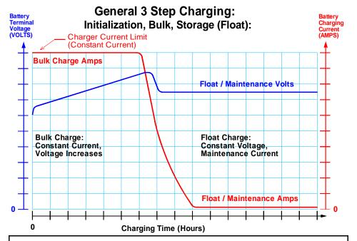
**Step 1) Initialization:** LED is Amber: Monitor Circuit verifies appropriate battery voltage levels and good electrical continuity between the battery and the charger DC output. If the AC power is connected and the LED remains OFF, check the DC connections to the battery.
