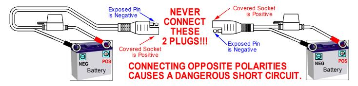
EVEN A RELATIVELY SMALL 18 TO 22 AMP HOUR MOTORCYCLE BATTERY CAN GENERATE SEVERAL HUNDRED, MAYBE EVEN MORE THAN ONE THOUSAND AMPERES WHEN THE TERMINALS ARE SHORT CIRCUITED!
