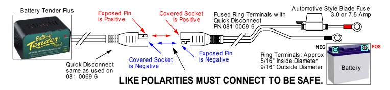
DANGER: NEVER CONNECT THE QUICK DISCONNECT PLUGS TOGETHER ON TWO (2) DC CABLE ASSEMBLY ACCESSORIES THAT ARE BOTH CONNECTED TO BATTERIES.
