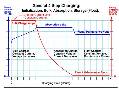
**Step 1) Initialization:** Red Light On: Monitor Circuit verifies appropriate battery voltage levels and good electrical continuity between the battery and the charger DC output.
